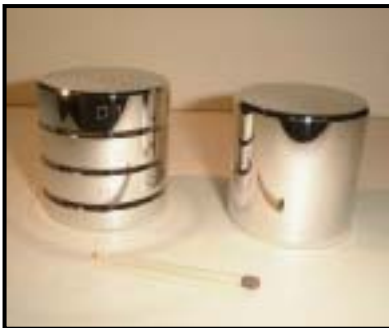
Two 1 kg Pt-Ir ( \Delta S = 77.8 \text{ cm}^2 )
