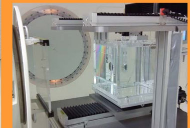
Ionization chamber in graphite jacket ...and water phantom.
