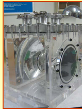
The calorimeter in its vacuum chamber.
