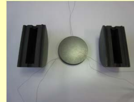
The design favours a homogeneous temperature distribution.
