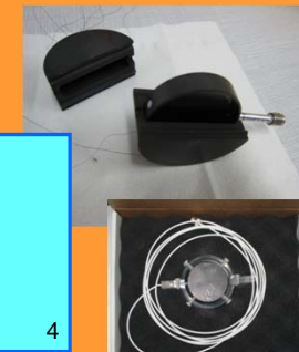
Ionization chamber in graphite jacket ...and water phantom.
